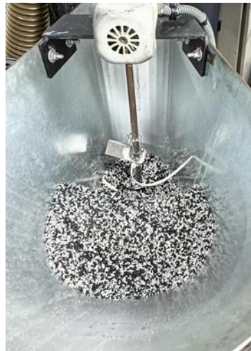
3 mm GRINDED EVA-RUBBER INSIDE THE SCREW PUMP
